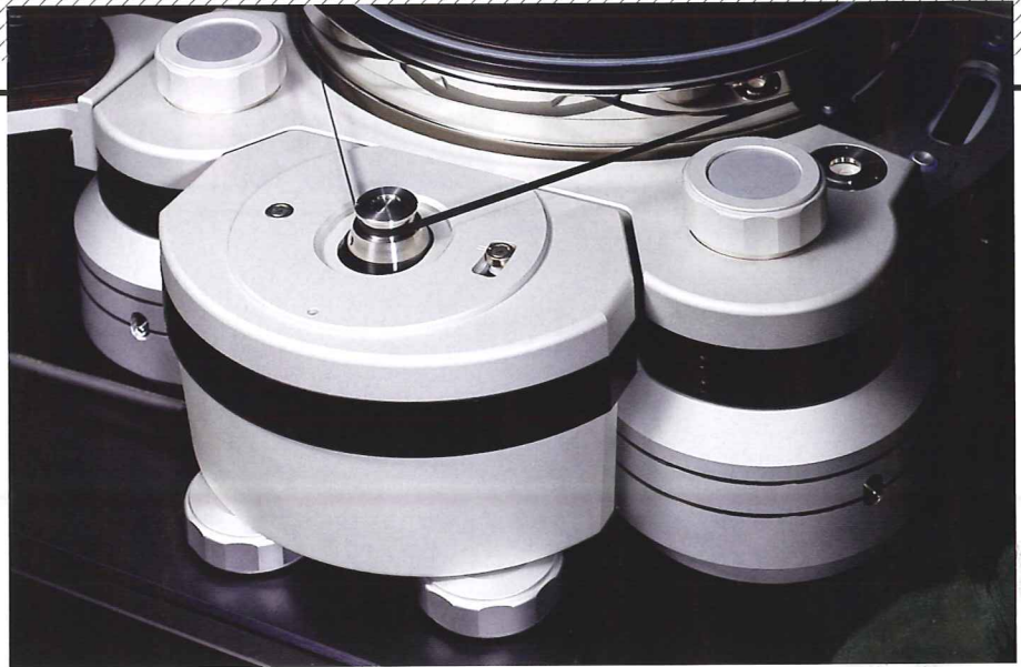
ABOVE: The huge AC synchronous motor is positioned adjacent to, but separate from, the main chassis. It is driven via a 2x50W amplifier for both phases and is adjustable in \pm 0.1 rpm steps
